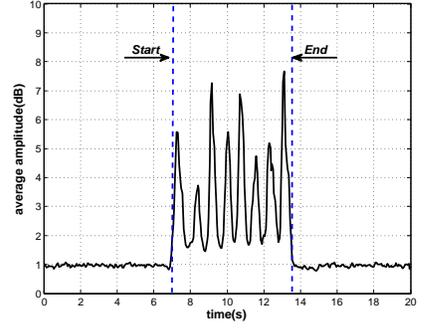
Fig. 7. The average amplitude of frequency bands except the pilot frequency during a 20 seconds driving containing a fetching forward event.
