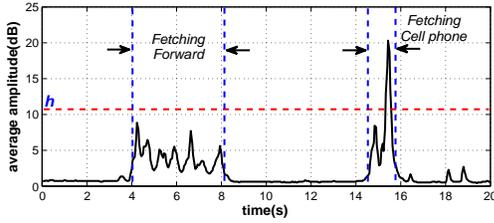
Fig. 9. The average amplitude of audio signals in 20 seconds driving containing a Fetching Forward event and an event of fetching smartphones.
