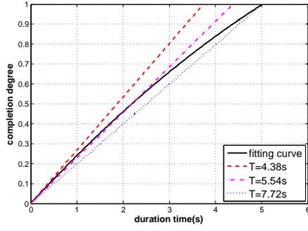
Fig. 5. The relationships between the completion degree  $\alpha$  and time duration  $\tau$  of fetching forward events under different the complete time  $T$ .
